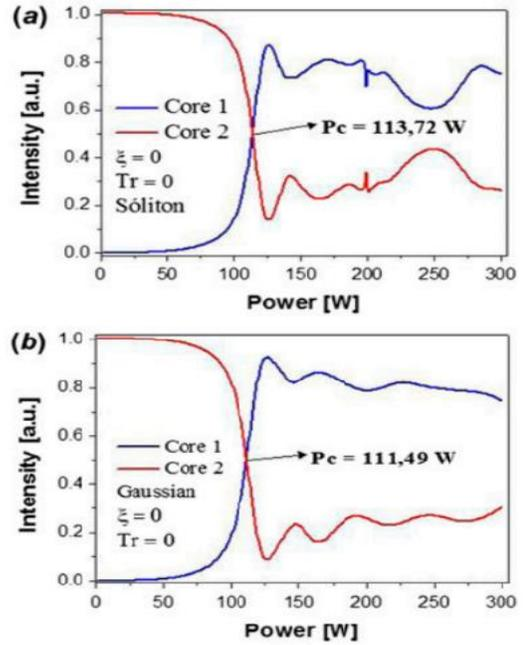
Fig. 1. The two types of pulses with no Raman effects (a) Soliton (b) Gaussian
