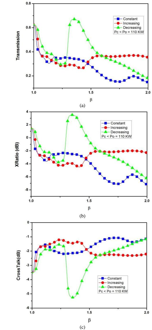
Figure 1: Results of the third scenario ( $P_0 = 110$  kW) considering the constant, increasing and decreasing profiles as for (a) transmission; (b) extinction ratio; (c) and crosstalk.
